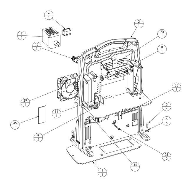
A-4.2, Main Structure Assembly 8LPM unit
