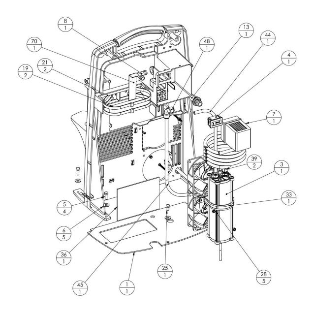
A-4.5, Main Structure Assembly 10LPM unit
