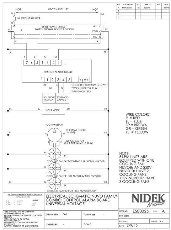
CAD FILE ES00025 Rev A, Electrical Schematic NUVO5,8,10 Combo
