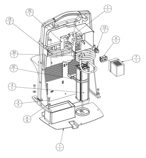
A-4.1, Main Structure Assembly 5LPM unit
